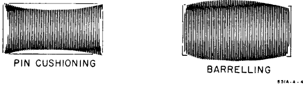
Figure 5-4. Pin-cushioning and Barrelling Defined
